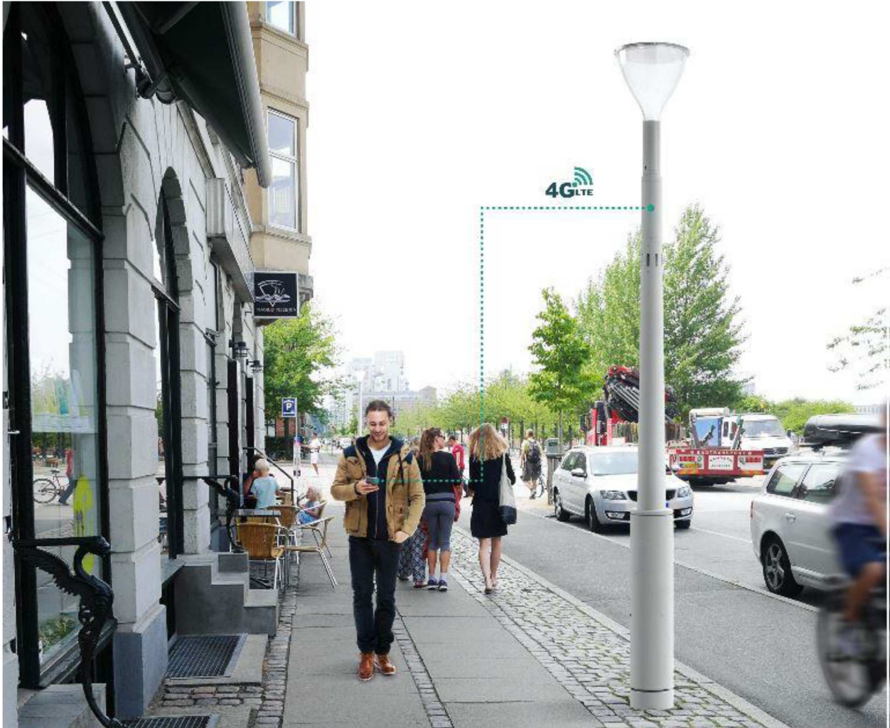
Exhibit 3. An antenna incorporated into, and hidden in the pole of top mounted, pedestrian scaled light may be acceptable if the light pole and fixtures matched those already existing or allowed in the City.
