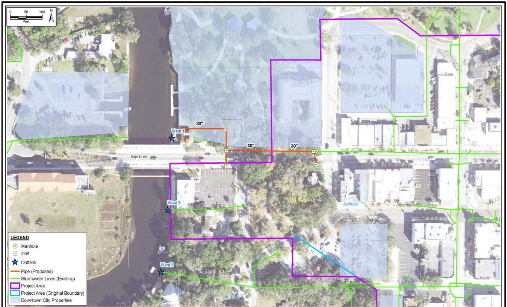
FIGURE 8. DRAINAGE AREA WEST-1 CONCEPTUAL PLAN DOWNTOWN REDEVELOPMENT AREA NEW PORT RICHEY, PASCO COUNTY, FLORIDA
