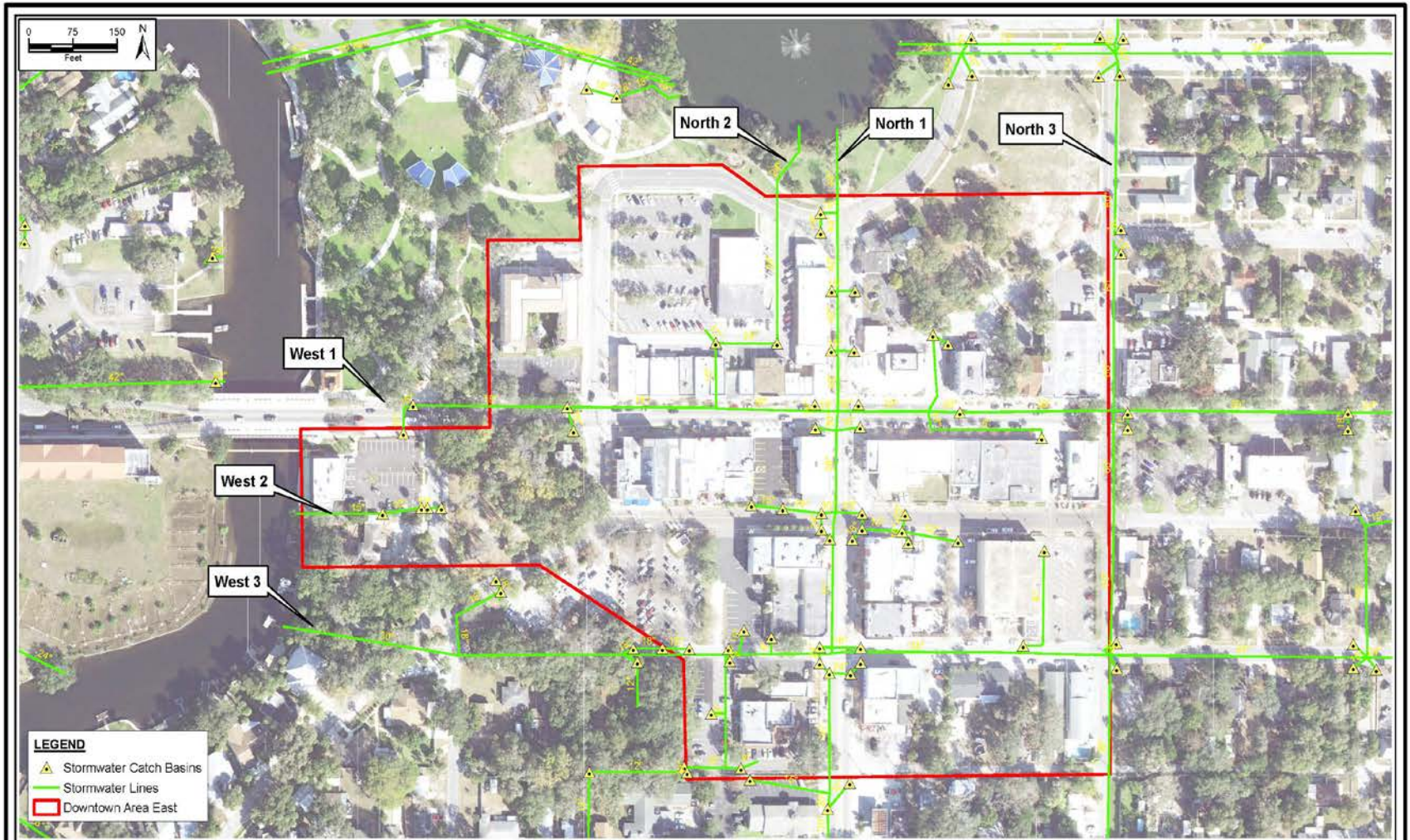
FIGURE 1. EXISTING STORMWATER SYSTEM LAYOUT DOWNTOWN REDEVELOPMENT AREA NEW PORT RICHEY, PASCO COUNTY, FLORIDA
