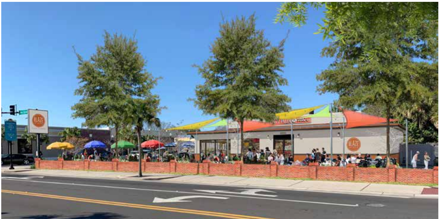
Option 5: The same as Option 4 except the buffer/edge to the sidewalk is achieved with a brick knee wall.
